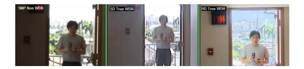
The worst is the SD, even though it is a true WDR. The 5MP non WDR beats it simply because it captures more details. Finally, the HD camera with true WDR performs the best.
