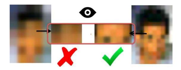
In the former image, the eyes were bigger than the pixels and therefore could not be captured. However, in the latter one, with pixels cover an area smaller than an individual eye, allows the eyes to be captured as two black dots.
