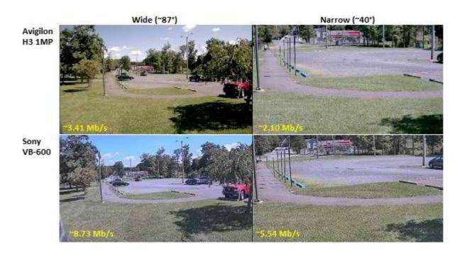
However, in a busy intersection/parking lot, bandwidth decreases by over 50% in the cameras below when widening the field of view. In the narrower FOV, more details of buildings are visible, and the repetitive pattern of the asphalt parking lot may be seen as well, making the scene more difficult to encode.
