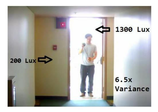
The WDR ratio is  $^{\sim}6.5x$ , with the open doorway at 1300 lux and the adjacent indoor sides at  $^{\sim}200$  lux.
