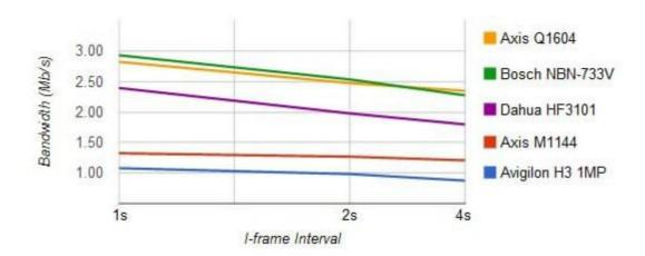
Inversely, increasing the number of I-frames to more than one per second significantly increased bandwidth, despite the minimal incrase in image quality.
